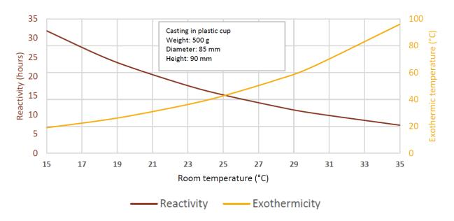
TriCast 50 Epoxy Resin System Reactivity vs time & temperature
