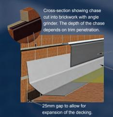
The C trim is fitted with PU adhesive applied to the back of the trim and is sealed into place with silicone sealant.
